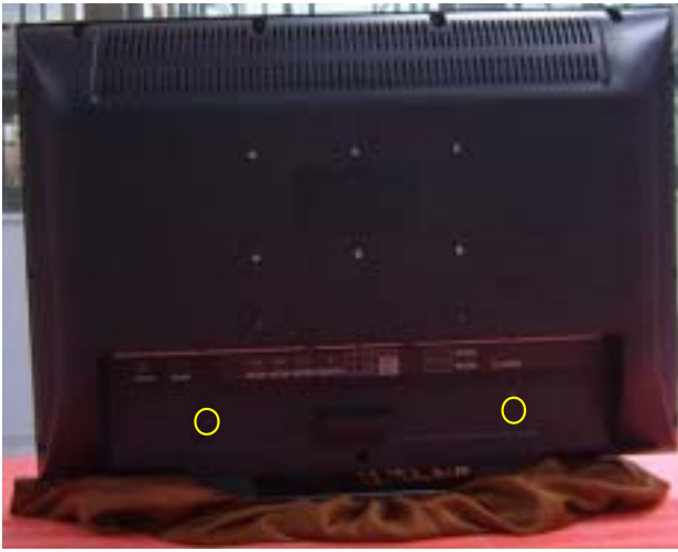
1. Release 2pcs screws and take off base.
