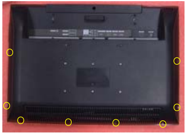
2. Release 8pcs screws from rear cover.
