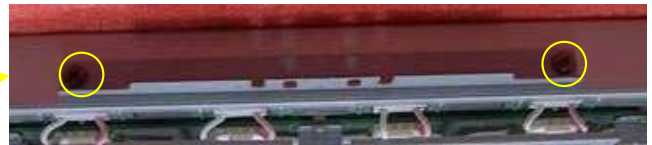
18. Release 5pcs screws from panel and take off bezel.
