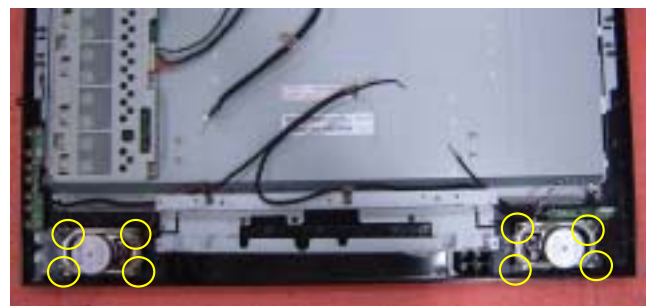
12. Release 4pcs screws from brackets.
