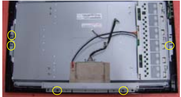
16. Release 3pcs screws from Button/B.
