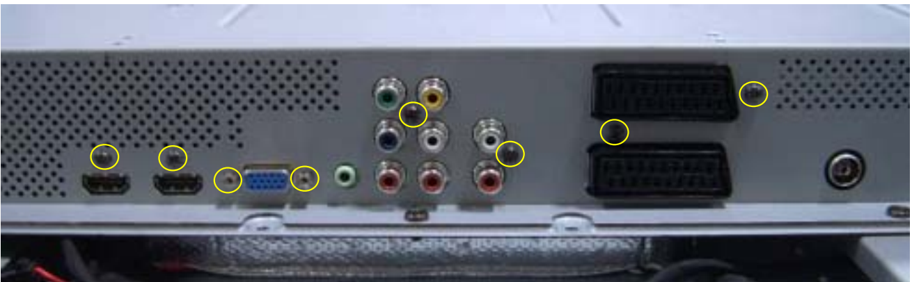
4. Release 8pcs screws from joint.
