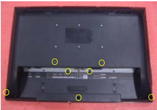
3. Release 7pcs screws from rear cover and take off it.
